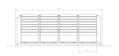
Portami bench with additional loose seats Steel supporting frame with permanently installed twin-seat bench and two loosely installed seats. - Length: 2.53 m - Weight: 98 kg
