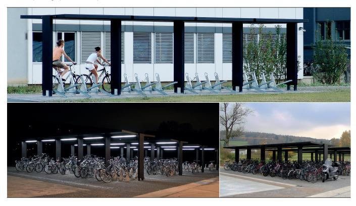
The covered bike racks were developed in connection with the Glattalbahn tram stop infrastructure. The racks can be extended in modules and offer space for 10 bikes in the Model 2 or 20 bikes in the Model 3.
