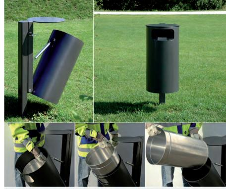
Public Bin (patent) provides the functional design for versatile deployment in parks and in the urban context. Public Bin 50L/110L can be opened easily from both sides. Thanks to an adjustable cushioning cylinder the bin tilts slowly into the removal position due to its high dead weight (3 mm stainless steel/CNS).
