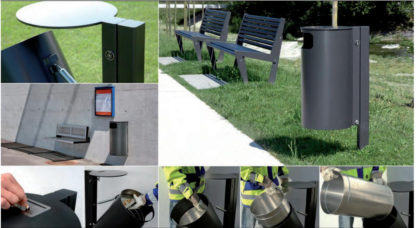
The powder-coated stainless steel 'Public Bin' with anti-graffiti surface can be opened easily from both sides. Thanks to an adjustable cushioning cylinder the bin tilts into removal position without pull due to its dead weight. The inner aluminium container can then be removed and emptied easily. Public Bin locks automatically when pushed back.
