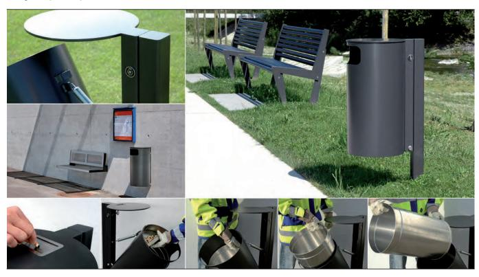
The powder-coated stainless steel 'Public Bin' with anti-graffiti surface can be opened easily from both sides. Thanks to an adjustable cushioning cylinder the bin tilts into removal position without pull due to its dead weight. The inner aluminium container can then be removed and emptied easily. Public Bin locks automatically when pushed back.
